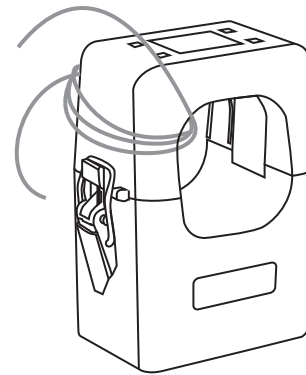
Figure 1: PDA6405 Current Transformer Shown with Four Turns
