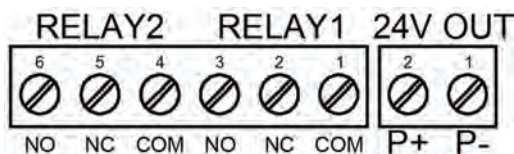
Figure 12. Relay & 24 V Output Connections
