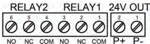
Figure 12. Relay & 24 V Output Connections
