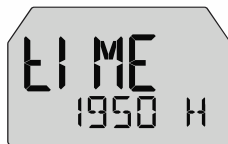
Meter displaying the amount of time a relay has been activated
