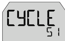
Meter displaying the number of times a relay has cycled
