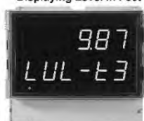
Local Display with PD2-6080 Master Displaying Level in Feet
