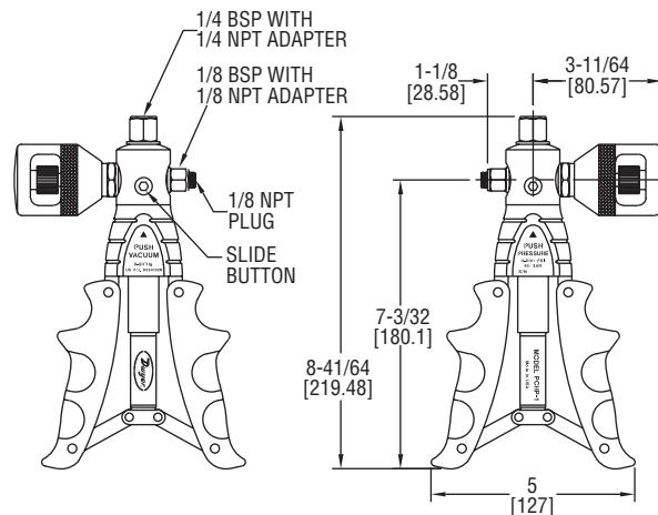
The **SERIES PCHP** Pneumatic Calibration Hand Pump sources pressure and vacuum to check calibration of gages, switches, transmitters, and recorders. The contoured cushion handles provide extra comfort while preventing the pump from sliding.
