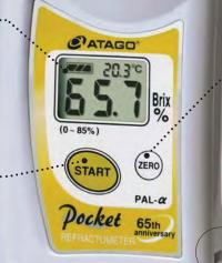
\* External Light Interference (ELI) - Patent Pending When intense light penetrates the prism of a digital refractometer, the light waves interfere with the sensor resulting in inaccurate readings. The PAL series is equipped with ELI technology, which will display the warning message "nnn" if the ambient light is too intense. If the warning message is displayed, simply turn away from the light source or shade the prism with your hand and press the START key
