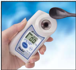
①Place the sample onto the prism surface.
