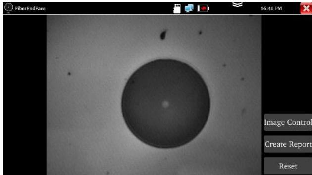
**It is used to inspecting the cleanliness of the fiber end face**
