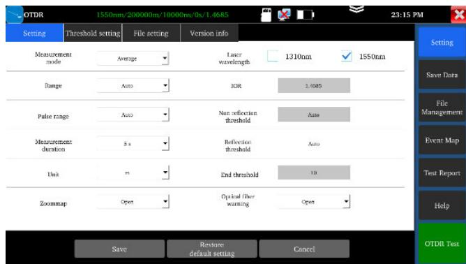
**Laser wavelength:** Selected by user, it provides several options, wavelength of single mode fiber: 1310nm, 1550nm and 1610nm. (If the fiber over 100KM, please select 1550nm wavelength for testing,
