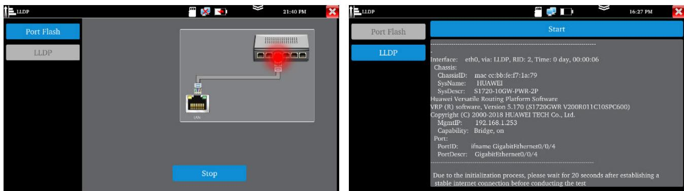
Quickly find the connected Ethernet cable
