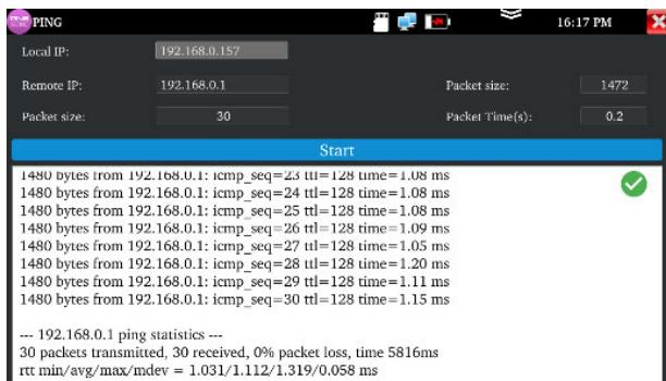
It is used for testing if the connected IP camera or other network equipment's Ethernet port is working normally, and the IP address is correct.
