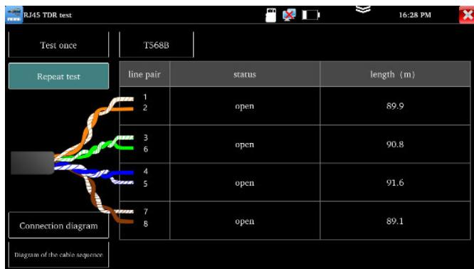
Connect cable to the LAN port of tester, the other end connects or disconnect other device. Enter "RJ45 cable TDR test" app to test cable's length.
