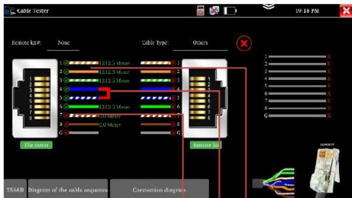
Test cable's continuity, length and fault locator of RJ45 cable connector. The number of the cable tester is 255. Connect LAN cable or telephone cable to UTP port of tester, the other end doesn't connect any device, can test fault locator of RJ45 cable connector and cable length. the other end connects to UTP port of wire receiver, enter cable test app to test cable's continuity and sequence.
