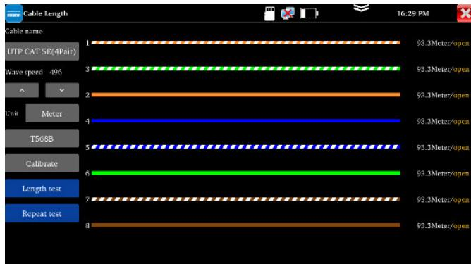
Note: The measured cable cannot be connected to any device. If connected to other devices, it will cause incorrect measurement results!
