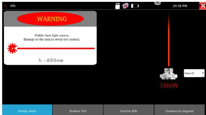
It is used to determine the continuity of optical fibers and locate faults
