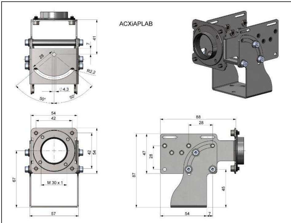
Figure 11: Mounting bracket (ACXIAPLAB), dimensions [mm], weight: 276 g
