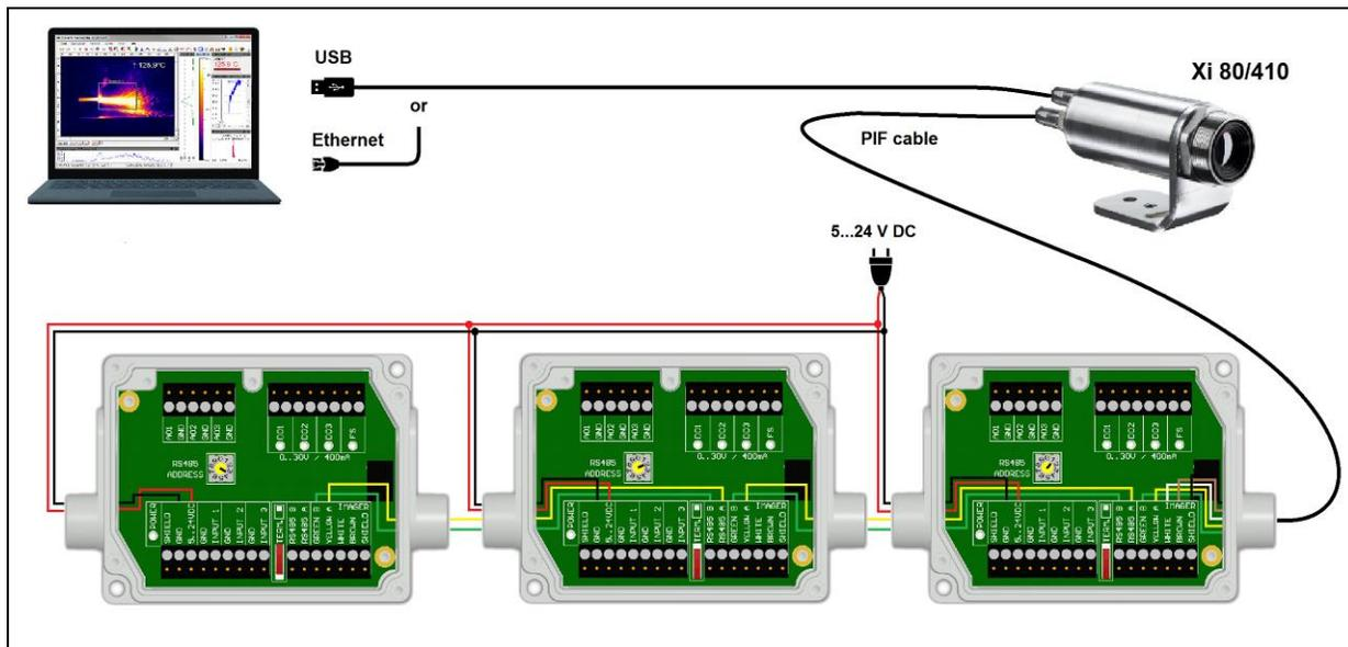
**Figure 30:** Connection of 3 industrial PIFs via RS485
