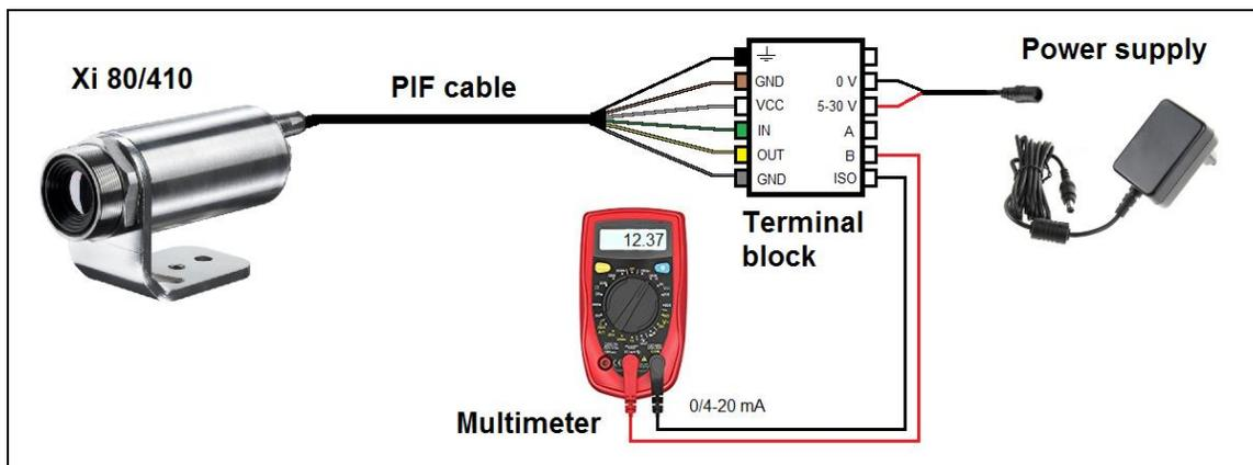
**Figure 40:** Electrical installation for autonomous operation Xi 80/410
