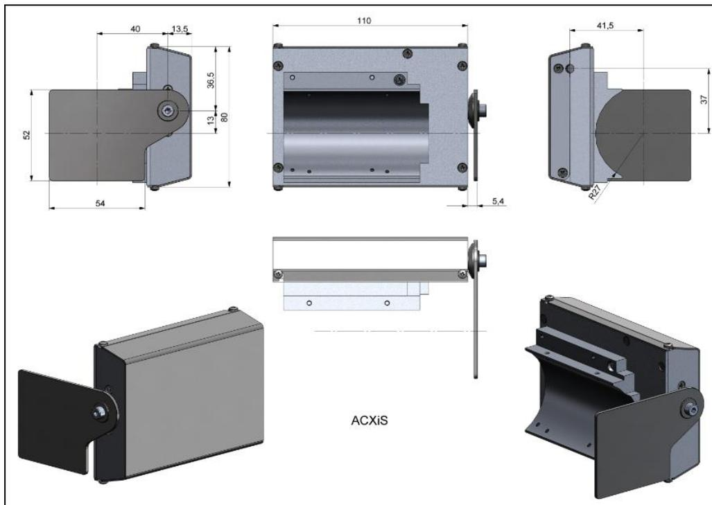
Figure 15: Shutter (ACXIS), dimensions [mm], weight: 550 g
