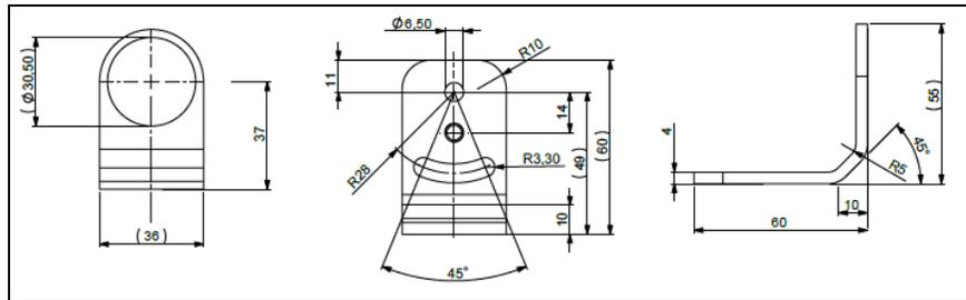
**Figure 4:** Mounting bracket, adjustable in one axis, with tripod thread
