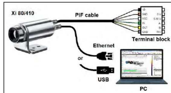
**Figure 36:** Connection Xi 80/410 to PC via Ethernet/USB
