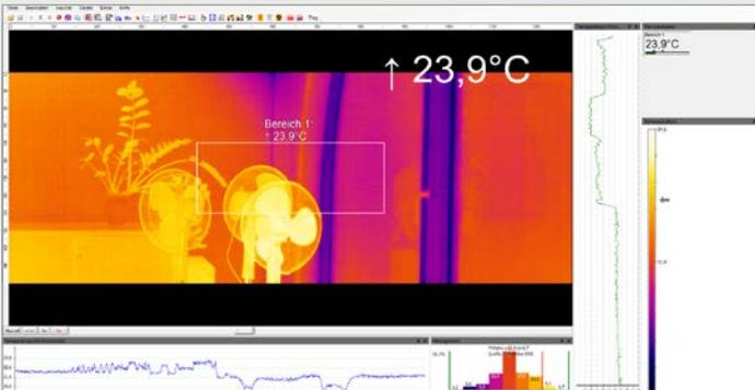
**The merging function combines several camera angles together in a single picture**
