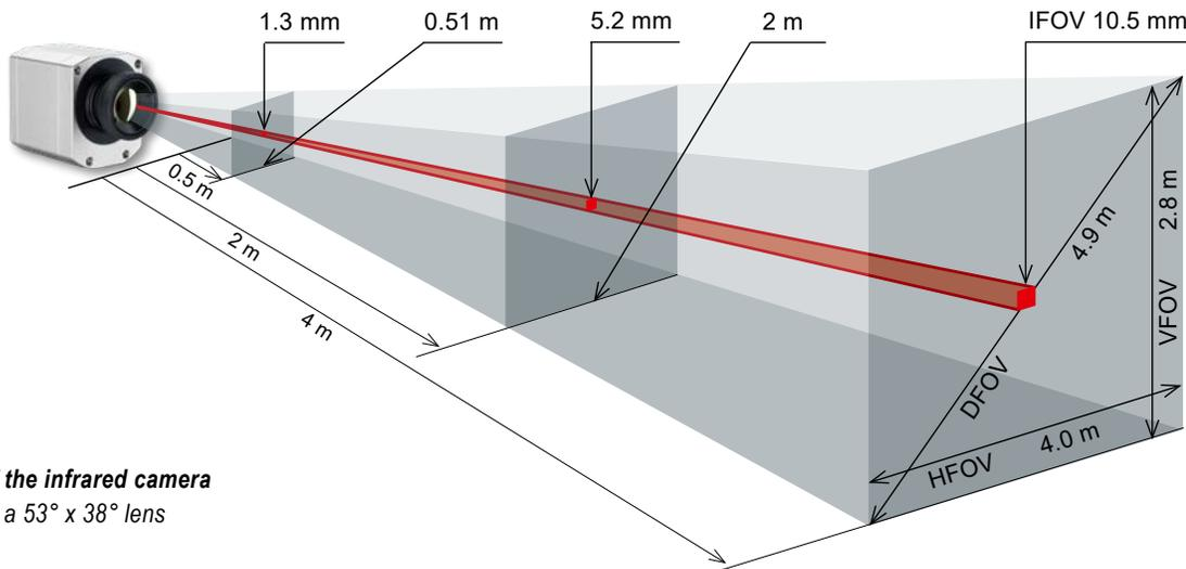
Measuring field of the infrared camera
