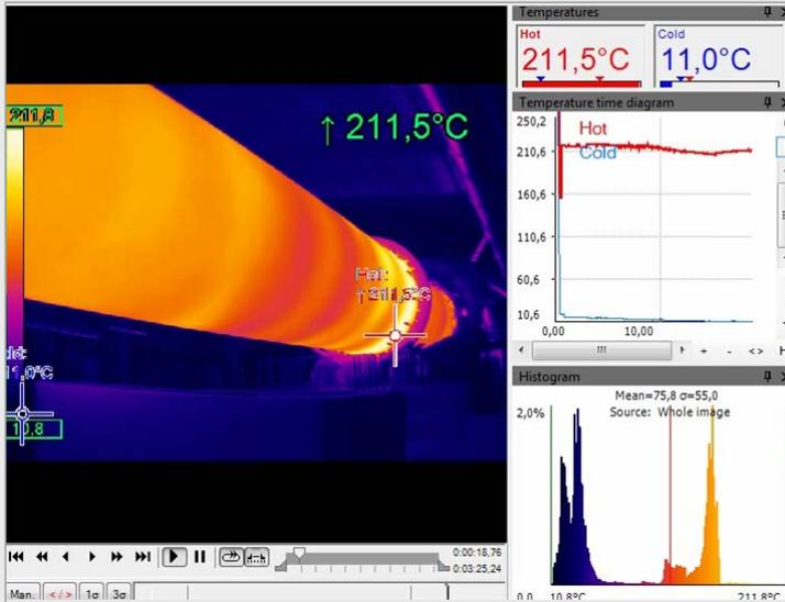
Beside of single snapshots also video recordings can be made with the software, both with radiometric data included. This allows a detailed analysis of the measurement results afterwards.
