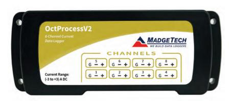
The OctProcessV2 is an 4-channel, battery powered, low level DC current data logger with a reading rate of up to 4 Hz. It can measure and record 32,736 readings per channel. To maximize memory capacity, users can enable or disable channels. For easy identification, each channel can be named with up to a ten digit title.
