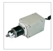
^ A Series R52 torque sensor is shown with the optional AC1014 Jacobs chuck attachment.
