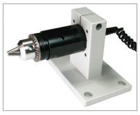
^ Optional AC1007 tabletop mounting kit may be used to hold the sensor in place.
