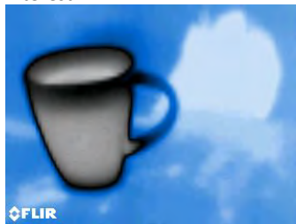
Fig. 5-7(a) Palette auto-scale unlocked
