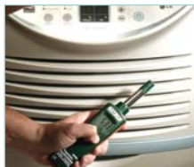
Precision Hygro-Thermometer with 2%RH accuracy and fast 30sec RH response time. Measures Humidity, Temperature, Dew Point, Wet Bulb, GPP and g/kg
