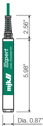
MJK Expert™ 1400 level transmitter
