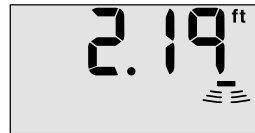
Example: Normal display read-out - none of the segments are flashing.
