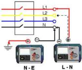
The insulation tests apply a known voltage to the circuit under test and measure the resulting leakage current.
