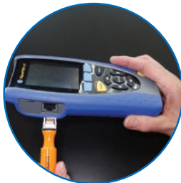
Replaceable RJ45 contacts
