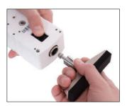
Attachments are mounted to the gauge's receptacle via the Click-Lock<sup>TM</sup> mechanism. Line up the attachment with the receptacle, and press in until a click occurs. The attachment may be inserted in 90- or 180-degree orientations. To release the attachment, pull back on the lever in the rear of the housing, as shown at left.
