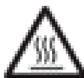
Caution, hot surface
