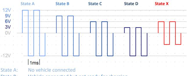
State B: Vehicle connected but not ready for charging State C: Vehicle ready for charging without ventilation State D: Vehicle ready for charging with ventilation
