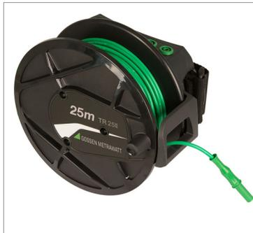
25 m measurement cable coiled onto a plastic reel. Connection to the inside end of the cable is made possible with two sockets integrated into the reel. The other end is equipped with a banana plug. Cable resistance can be compensated for with the rotary selector switch in the R<sub>LO</sub> position.
