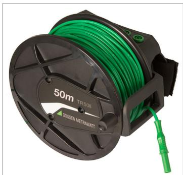
50 m measurement cable coiled onto a plastic reel. Connection to the inside end of the cable is made possible with two sockets integrated into the reel. The other end is equipped with a banana plug. Cable resistance can be compensated for with the rotary selector switch in the R<sub>LO</sub> position.
