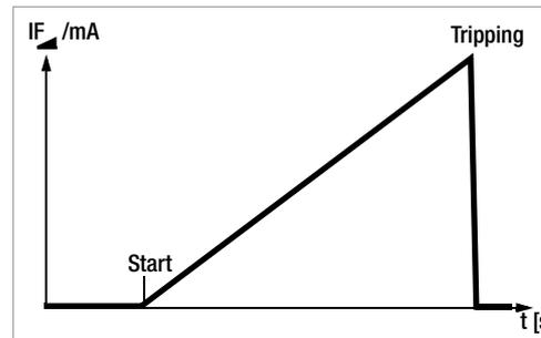
With the selector switch in the  $I_F$  position, slowly rising DC current flows via N and PE. The momentary measured current value is continuously displayed. When the RCCB is
