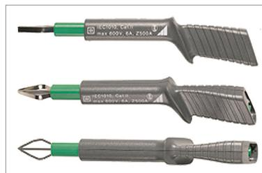
Three self-retaining test probes with touch protection for the connection of measurement cables with 4 mm banana plugs, or with touch protected plugs for sockets with an opening of 3.5 mm to 12 mm, e.g. CEE or Perilex sockets etc.
