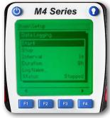
Data Logging is standard on all M4 models. Select Data Logging from the Setup key menu and then enter the desired Interval and Duration parameters using the keypad controls. For M400 single pressure sensor units, pressure, VDC and mA DC values are saved to the SD card at each interval. M402 dual pressure sensor units log both pressure values plus VDC and mA DC values.
