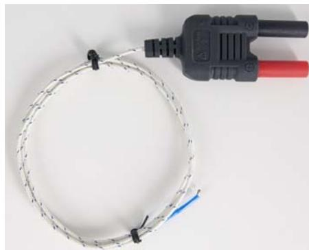
Type K thermocouple with banana plugs
