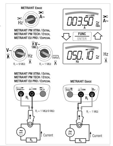
5.7.5 Direct, Pulsating and Current Measurement with Current Clamps
