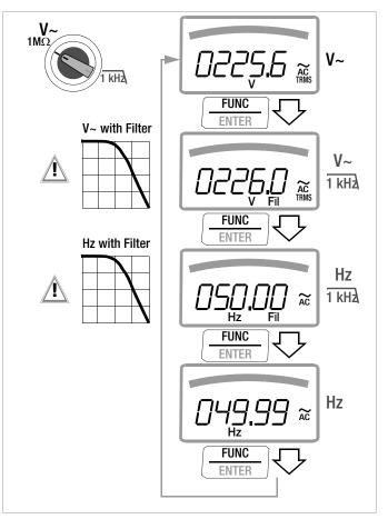
5.1.3 Alternating Voltage and Frequency Measurement V AC and Hz with Selectable Low-Pass Filter (METRAHIT AM X-TRA / AM TECH / AM PRO / X-TRA / OUTDOOR / TECH / PRO / SECULIFEHITAM/MD only)
