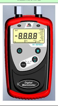
Meriam Process Technologies' M1 Series pressure instrument is a microcontroller-based pressure sensing device that can be used to directly measure pressure. Differential, Gauge and Absolute pressure sensors are supported up to 100 PSI. Pressure can be displayed in selectable engineering units of PSI, bar, mbar, kPa, mmHg, inHg, mmH2O or inH2O.
