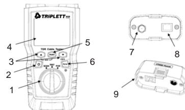
1. Mode knob: Wire tracking mode, testing mode, POE mode
