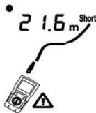
Figure 6.16 Short on Coaxial Cabling
