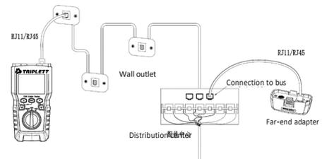
Figure 6.12 Connecting to Telephone Networks in Bus Topologies
