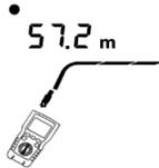
Figure 6.15 Open on Coaxial Cabling
