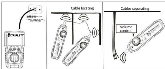
Figure 8.2 Wire Tracking Diagram
