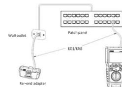
Figure 6.1 Connecting to Twisted Pair Network cabling
