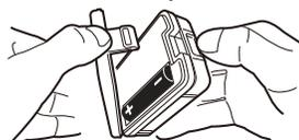
*Note. With the LR5001, recording is interrupted during battery replacement if the battery is very weak. After batteries are replaced, recording resumes automatically. Previously recorded data is not lost during battery replacement.*
