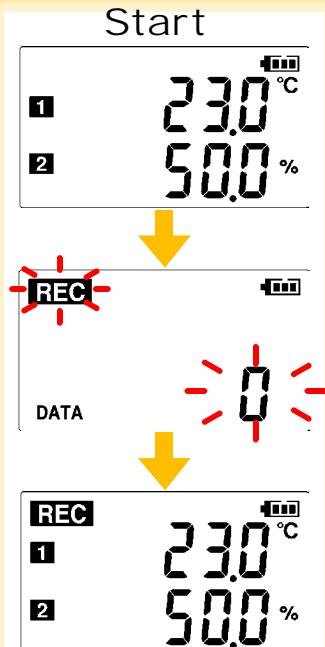
**Start** From the Measurement display, hold the **REC/STOP** button for two seconds.
