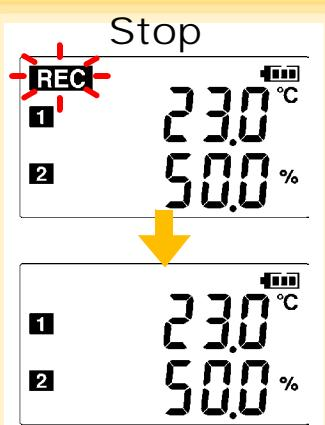
**Stop** Hold the **REC/STOP** button for two seconds while recording (while **[REC]** is displayed).
