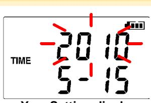
1 Press the **SET** button to display the time settings. (**[TIME]** is displayed, and the year setting blinks.)
