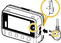
2 Connect the LR9504 Humidity Sensor to the logger.
