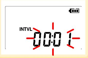
1 Press the **SET** button to display the interval setting. (The **[INTVL]** indicator appears, and the setting blinks.)
