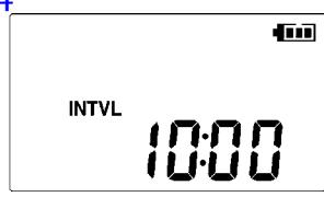
4 Select the recording interval for the logger (in this case, 10 minutes).
