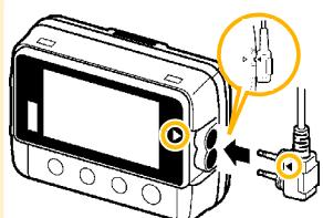
Align the triangle on the plug with the one in front of the sensor jacks, and insert the plug securely.
