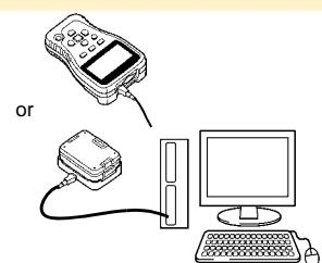
1 Plug the USB cable into the USB port on the LR5091 (or LR5092-20), and into a USB port on the computer.
