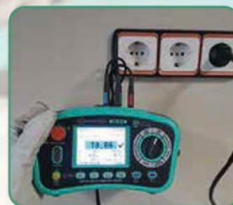
Loop test from a wall socket
