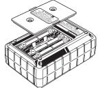
Install batteries in correct polarity as marked inside.
