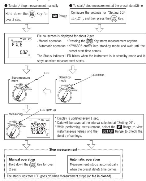
\* When the destination to save data has been set to the internal memory, "嵊颠" symbol is displayed on the screen instead of "函" symbol.
