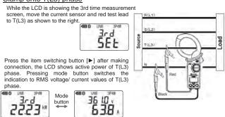
Another press of item switching button [▶] switches the screens to measurement result.
