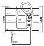
Press the item switching button [▶] after making connection, the LCD shows active power of R(L1) phase. Pressing mode button switches the indication between active power of R(L1) phase and RMS voltage/ current values.
