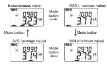
Range is fixed while the LCD is showing MAX, MIN, or AVG. The auto-ranging function is reactivated when switching the display to instantaneous value.
