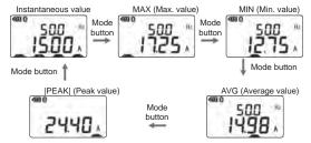
Range is fixed while the LCD is showing MAX, MIN, AVG, or |PEAK|. The auto-ranging function is reactivated when switching the display to instantaneous value.
