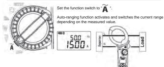
A short press of Mode button: switches display modes between Inst, MAX, MIN, AVG, and |PEAK|.
