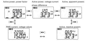
Mode button Short press: switches display modes between Inst, MAX, MIN, and AVG.
