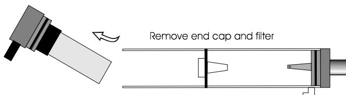
Remove the end cap from the in-line filter housing. Carefully remove the paper filter element and dispose of it. Clean the inside of the filter housing with a suitable soft cloth. Insert a new filter element onto the spigot in the filter housing and carefully replace the end cap.
