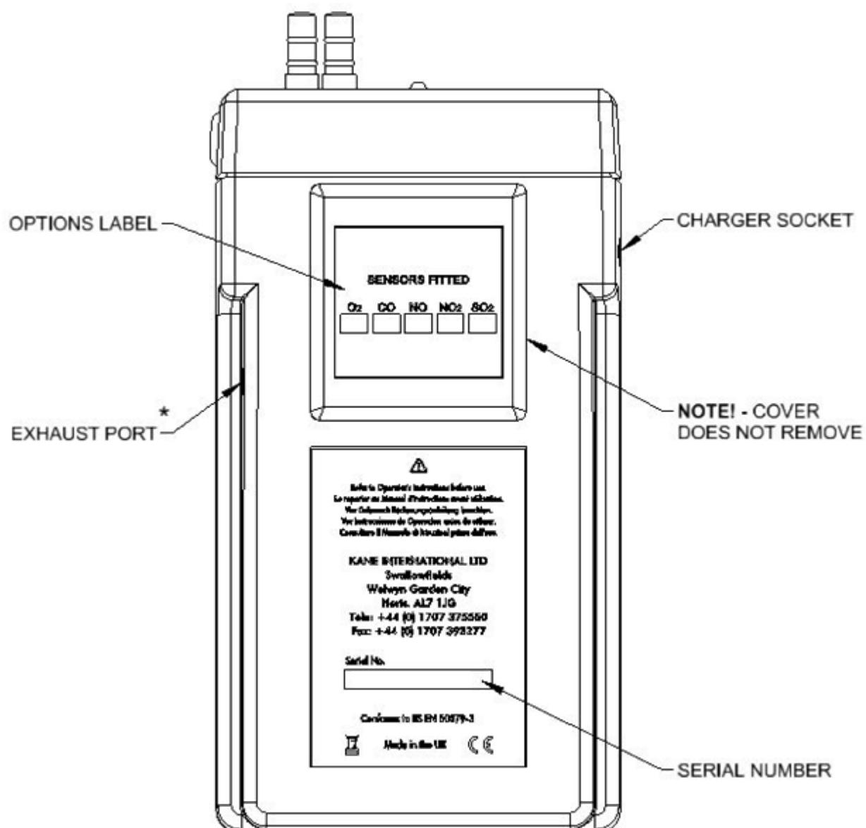
**NOTE:** Do NOT cover exhaust port as this will severely affect analyser operation
