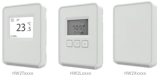
The HW2 Series of humidity sensors for living space is a flexible multisensor platform for use with BAS controllers designed to accept 4 to 20mA, 0 to 5Vdc or 0 to 10Vdc outputs. HW2 Series sensors are available with three user interface options: touchscreen, LCD with three buttons and blank. Humidity and temperature sensors are included with all HW2 Series sensors.
