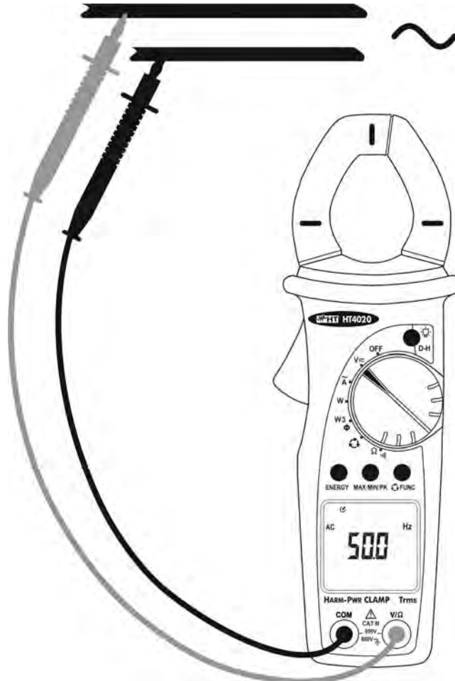
Fig. 5: Use of instrument for AC voltage frequency measurement
