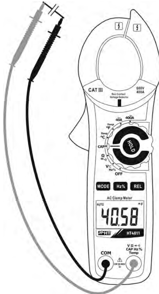
Fig. 6: Use of the clamp for capacitance measurement
