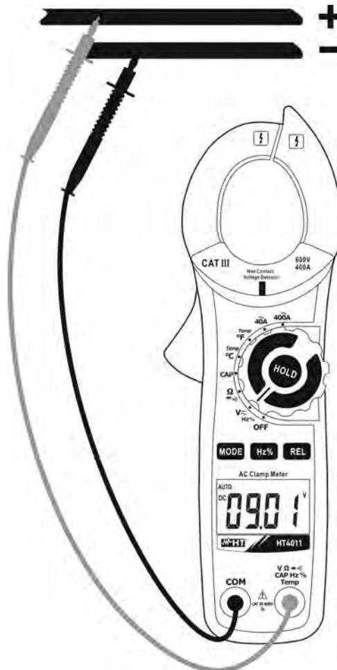
Fig. 2: Use of the clamp for DC voltage measurement
