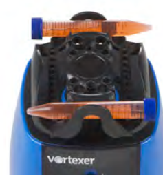
15 mL conical tubes x 2 (horizontally mounted)
