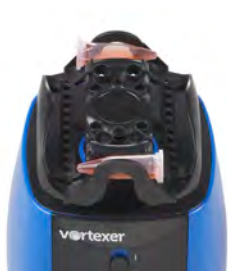
5 mL tubes x 2 (horizontally mounted in the same retention space as 15 mL)
