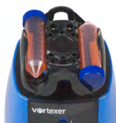
50 mL conical tubes x 2 (horizontally mounted)
