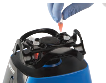
1.5/2 mL microfuge tubes x 4 (vertically mounted)
