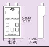
The Series HM28 Digital Hand-Held Manometer is a precision instrument designed to measure a wide range of pressures to a very high accuracy. The unit incorporates a variety of features in an easy to use format that makes it useful in a wide variety of applications. Features include: measurement in all common pressure ranges, display resolution to 0.001, differential or relative measurement, two line liquid crystal display, and adjustable auto power off to conserve battery.
