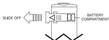
Batteries should only be replaced in a nonhazardous area using the battery type specified in this instruction manual.
