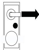
The cloth junction can be pulled out approximately 20 times. After that, the electrode should be replaced.
