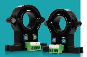
The HAK Series Hall effect DC current sensors provide precision measurements of DC current up to 200A with a standard 4-20mA or 0-5V output signal for broad compatibility. Featuring a hinged split-core design for fast, easy installation into existing systems, the HAK provides accurate 0.5% measurements for any DC project and is available as either a unidirectional or bi-directional device.
