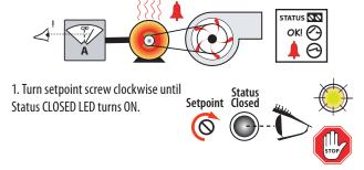
2. Slowly turn the setpoint screw counter-clockwise until the Status OPEN LED just turns ON.
