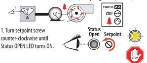
2. Slowly turn the screw clockwise until the Status CLOSED LED just turns ON.
