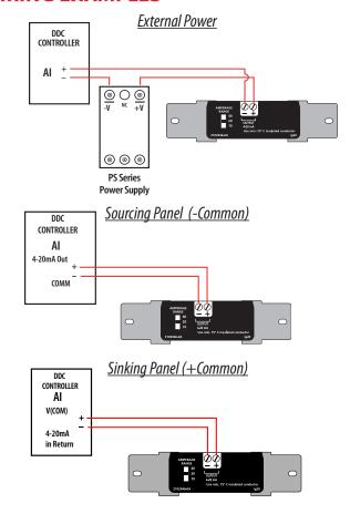
\*A resistor can be added in parallel to convert the 4-20mA signal to a VDC signal (250 ohm= 1-5VDC); (500 ohm = 2-10VDC)
