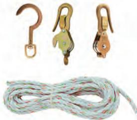
All Klein block and tackle use high-quality, 3/8-Inch (10 mm) diameter rope. Light, galvanized-steel shell blocks are fitted with snubbing hooks to hold the load. This package features two blocks with a swivel Klein hook Cat. No. 259 with a maximum safe load of 750-Pound (340 kg).
