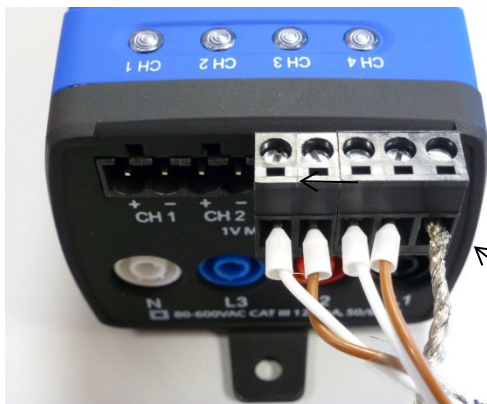
Connecting RōCoil CTs to an ELITEpro XC
