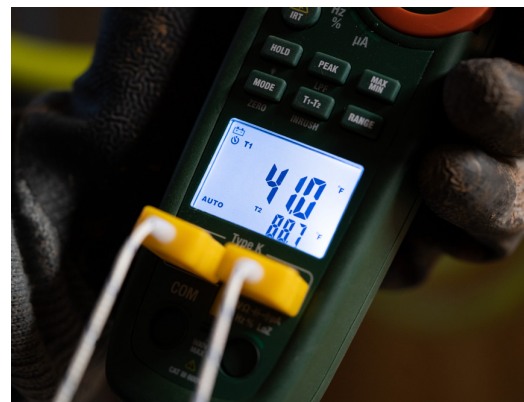
Dual Type K thermometer for taking differential temperature readings needed for superheat measurements.
