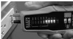
Measuring above 240V should be limited to 30 seconds continuous, followed by a recommended recovery time of at least 240 seconds (4 minutes).
